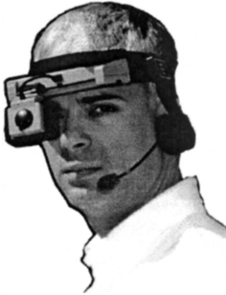
Figure 1. Kopin headset used in 1997 study of the feasibility of wearable EPSSs ( http://mime1.gtri.gatech.edu/MiME/papers/ISWC_Jenn.html ).
